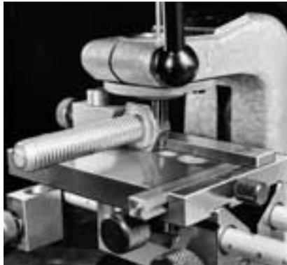
Reglus drilling jig in use: special drill bushes facilitate the drilling of security holes in hexagonal material.
